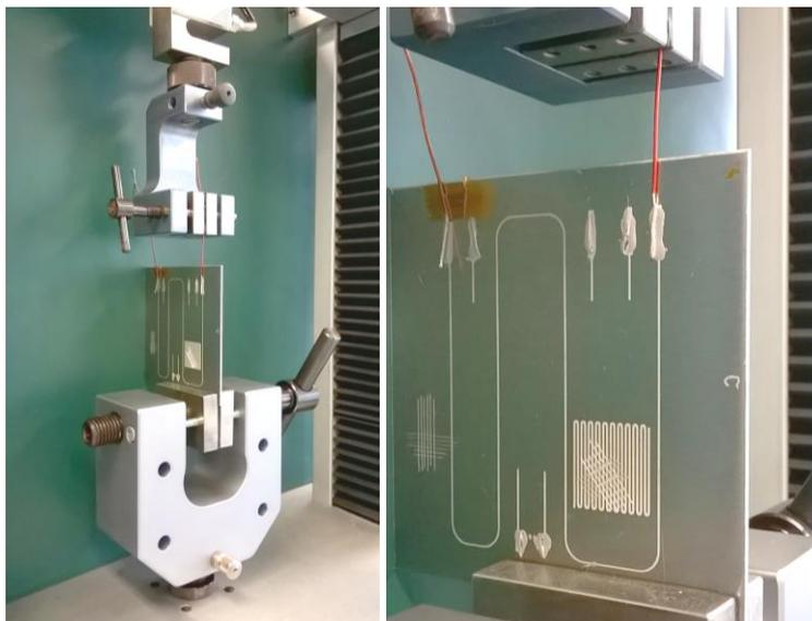
Fig. 9. Aluminium sheet with wiring in tensile testing machine for determination of lead-pull strength.
