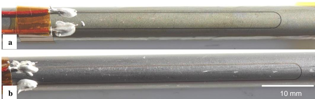
Fig. 3. Titanium alloy tubes with aerosol jetted and contacted heating tracks of a) 80 mm length on polyimide coating, b) 100 mm length on IFAM plasma coating.
